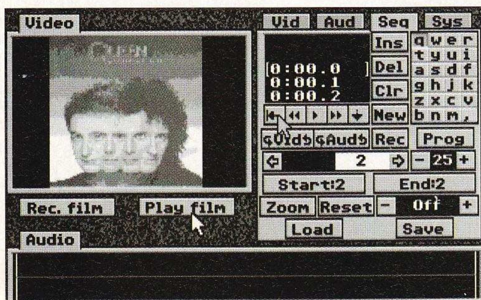
VideoMaster grabs live video footage with sound at up to 25 frames a second on any ST.
